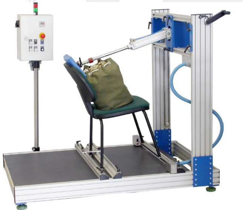
40-930-080 Test rig for tilting drop testing of fourfeeter indoor and office chair as well as outdoor furniture stool and cantilever chair (freeswinger chair) in acc. to DIN 68878.
