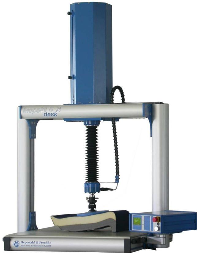
10-012-907 Special test machine for foam compression test e.g. in acc. to DIN 53579 and ISO 2439 (hardness evaluation on foam products and fabricates), ASTM D 3574-B1 (firm hardness) and EN ISO 3386-1 (determination of deformation properties)
