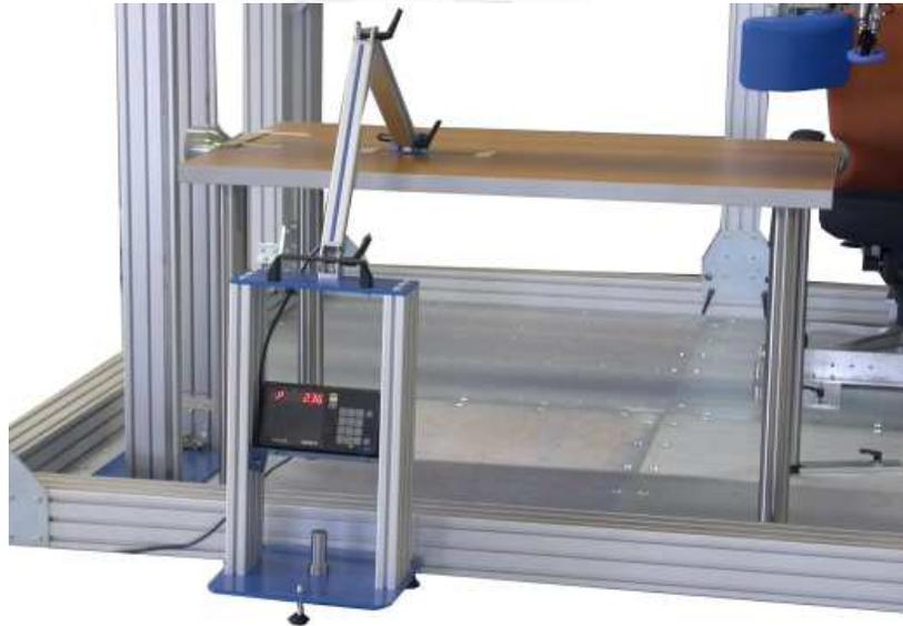
**LEFT:** 41-002-200 Pendulum impact test station, e.g. acc. EN 581, EN 716, EN 1130, EN 1153, prEN 518, EN 1728, EN 12221, EN 12227, EN 12727, ENV1178 incl. A set of three impact hammer:
