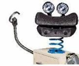
...standard conform alternating bending testing at seat/backrest of office chair
