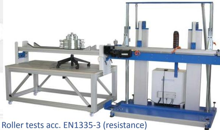
Roller tests acc. EN1335-3 (resistance)
