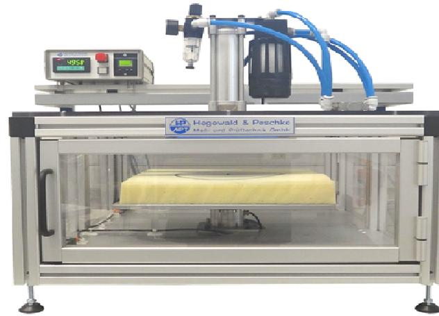
41-026-023 fatigue testing of foams in acc. to DIN EN ISO 3385 (constant rate of compressions, 70 hits a minute up to 750N, 80,000 cycles – can be varied)
