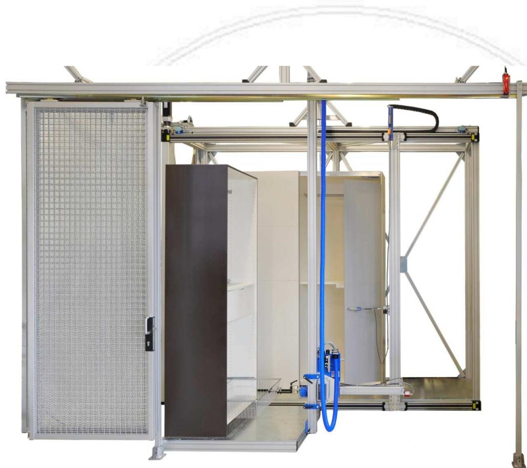
Combined test rig for revolving and sliding doors as well as for drawer
