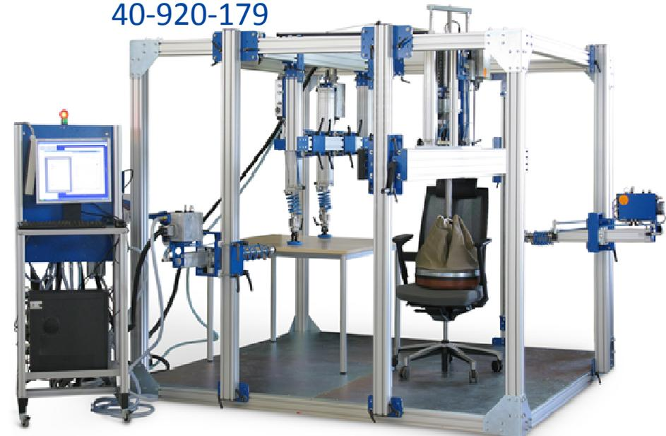
Universal test rigs with a static optimized and solid test frame and strong galvanized base plates with a thread pattern for easy and flexible fixation of specimen.
