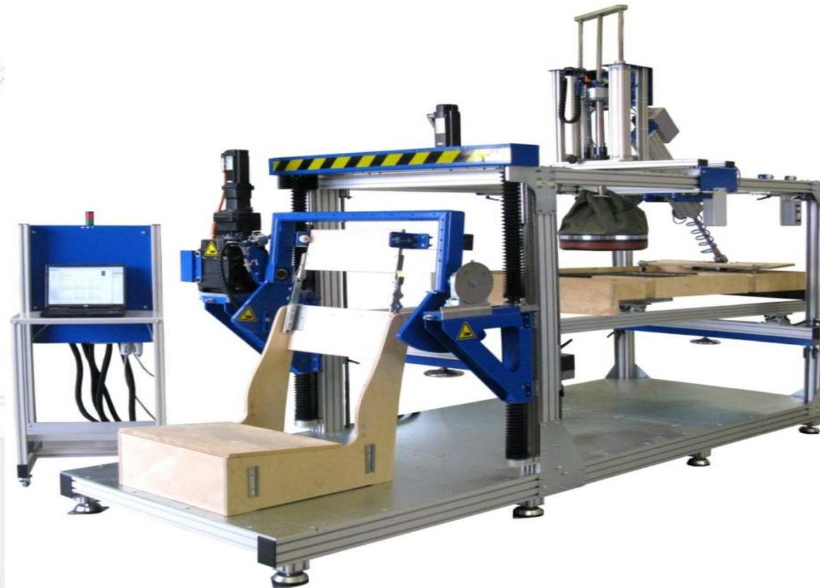
„One for All“: With that special test structure all mechanism on a cushion frame are tested. The head rest of sofa frames is rotated and arrested in different lock positions as well as the head rest of bed frames. Additionally the unit contains a drop tester.
