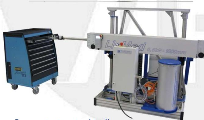
Drawer test on tool trolleys
