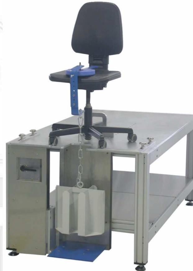
40-910-090 Stability test on chair and seating furniture acc. to EN 1022, EN 1729, EN 581-2-3, EN 1335, DIN 68878 and BIFMA X 5.1
